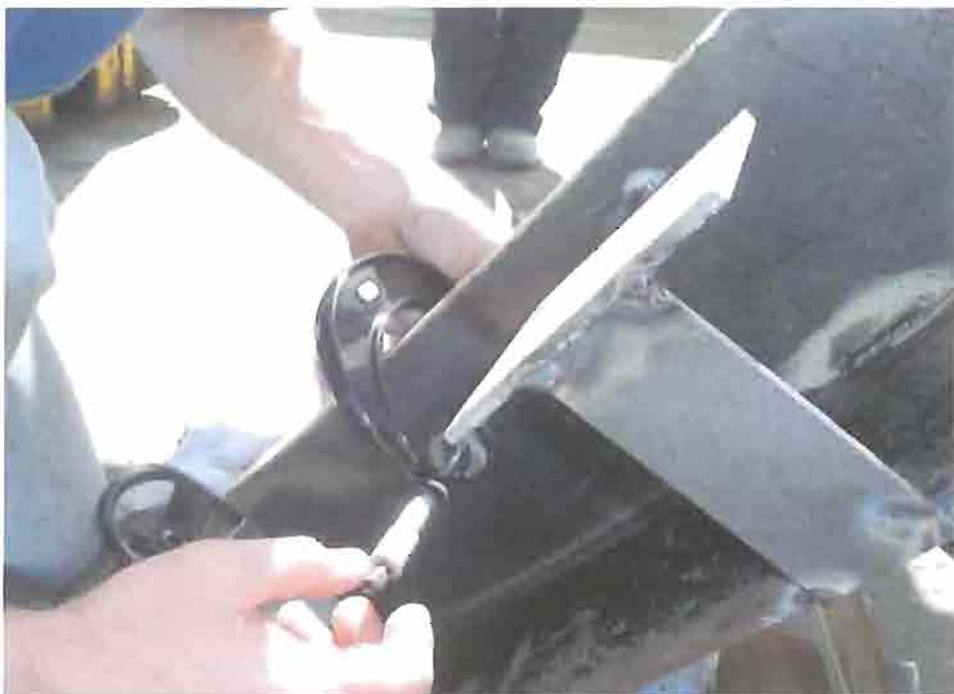
Figure 2. Bolt length measured under load
