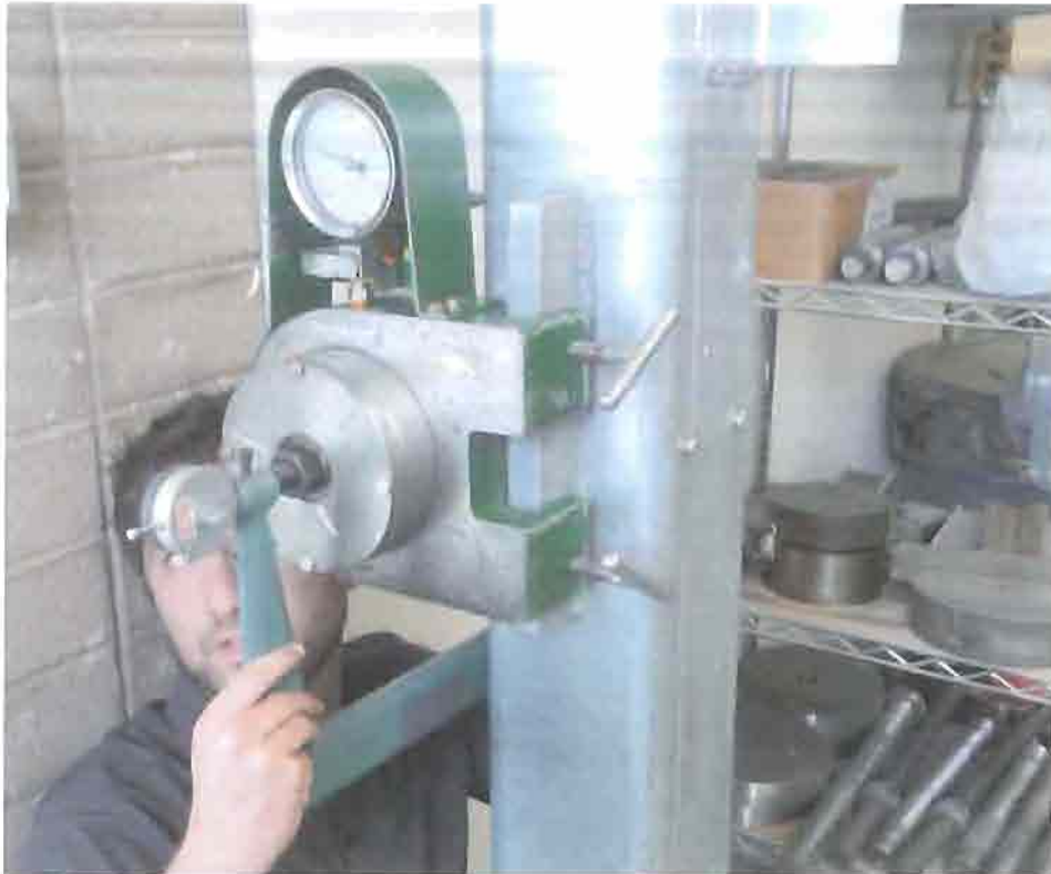
Figure 4. Measuring bolt length under load using special caliper
