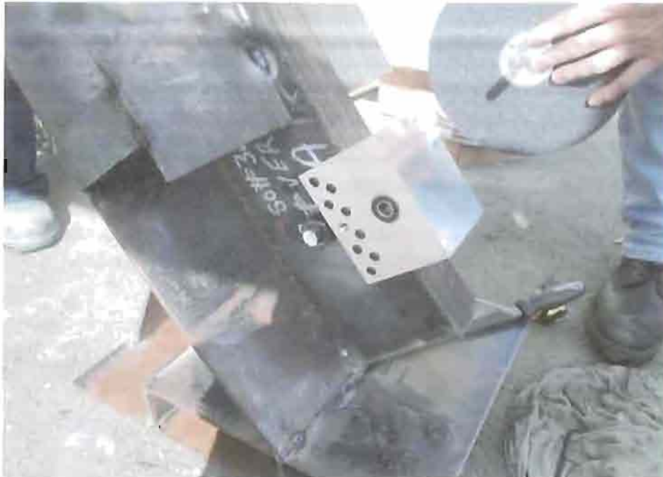
Figure 1. Mock up assembly with installed bolt and machining fixture
