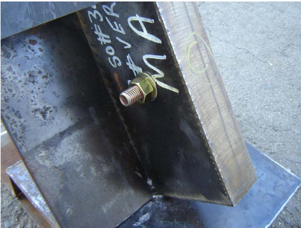
Simulated shell plate, structural Tees and floor at location "C"
