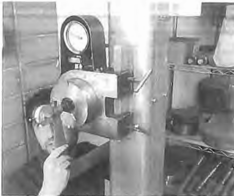
Figure 4. Measuring bolt length under load using special caliper
