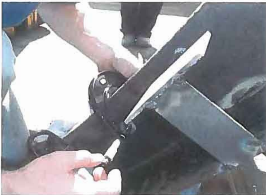
Figure 2. Bolt length measured under load
