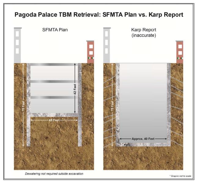
As planned, the secant piles will be drilled to a depth of approximately 25 feet below the depth of the retrieval shaft, which should block most, if not all, ground water from the excavation. Any water that might seep in would be minimal and would be removed without impact to surrounding properties.
